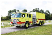
E 2000 GPM Pump, 4000 Gallon Tank, Light Tower, Only 3.....
