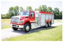
Hale 1500 GPM Pump, 2500 Gallon Tank, Cummins Diesel
