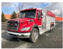
Waterous 1500 GPM Pump, 3000 Gallon Tank, Detroit Diesel
