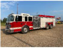
Hale 1500 GPM Pump, 2500 Gallon Tank, Cummins Diesel
