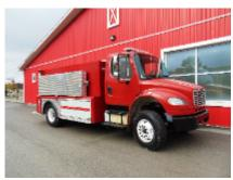
2000 Gallon Tank 350 GPM Pump, Cummins Diesel
