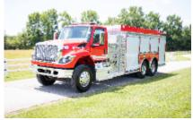
Hale 1500 GPM Pump, 2500 Gallon Tank, Cummins Diesel
